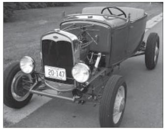
tube of 4130 steel was welded between the front horns. The steel roadster body, by Brookville, is a 1931 Roadster Pickup cab with six additional inches behind the doors. The gas tank is from the original Fordor.
